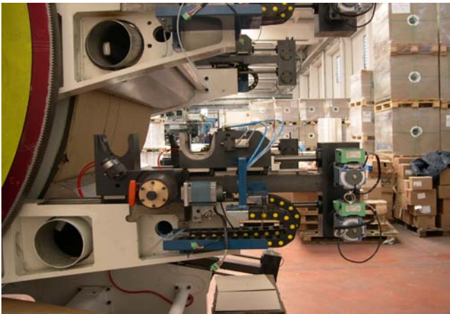
4-AC Motor And Ball Screw Design Deck Movement
