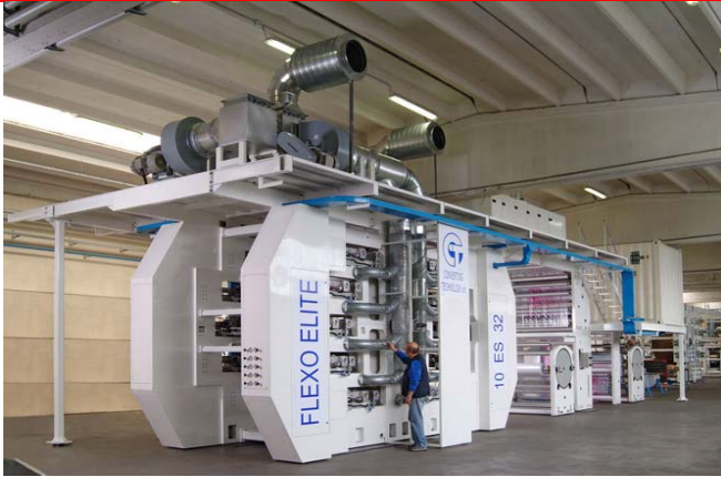
Doors And Guards Not Installed
